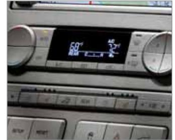
Dual-zone Electronic Automatic Temperature Control automatically maintains the selected temperature settings.
